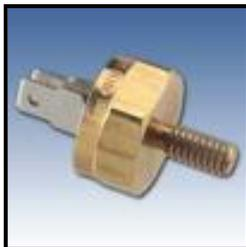
Simply Install in the engine coolant line, or into the port on the VegMax2 filter. Switch to SVO as soon as you get in the car and start the engine and the system will not change to SVO, nor turn on the VEG-Therm (if desired) until the coolant temperature reaches ~ 50 deg. C.
