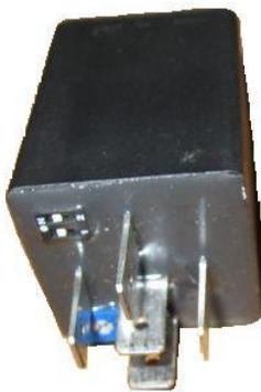
This is a microprocessor-controlled timer relay which is adjustable from seconds up to one hour. It can be used in a negative earth 12V DC or 24V DC system and will plug into a standard automotive relay base. The MFT purge timer can supply current up to 10 amps, so it can for example, control a Pollack 6 port motor drive valve, as well as controlling 3-port valves.
